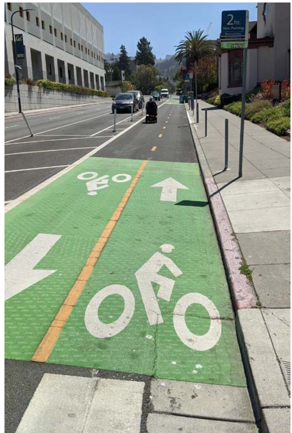
Two-way separated bikeway at Bancroft and Ellsworth.
